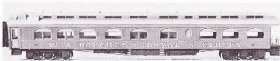
WOODEN SLEEPER OF THE TYPE USED BY THE MAJORITY OF SHOWS DURING THE ERA OF CIRCUS TRAINS.
