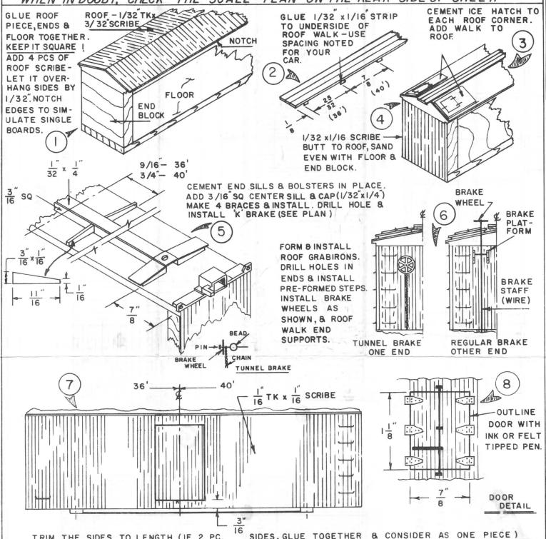
TRIM THE SIDES TO LENGTH (IF 2 PC. SIDES, GLUE TOGETHER & CONSIDER AS ONE PIECE) COVER THE END SHEETING. OUTLINE THE DOOR AS NOTED. CEMENT HINGES & LATCH BAR IN PLACE AS PER DOOR DETAIL. DRILL HOLES AND CEMENT PRE-FORMED GRAB-IRONS IN PLACE. ADD CARD STOCK DESTINATION BOARDS. IF UNDECORATED, DECAL FOR YOUR ROAD. INSTALL
